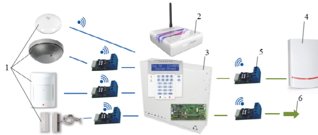
Fig. 2. Integration model: 1 – loop detectors; 2 – Fibaro HC Lite (only monitoring features); 3 – loop switchboard with case and keypad; 4 – loop alarm; 5 – Fibaro Universal Binary Sensor; 6 – free PGM outputs
