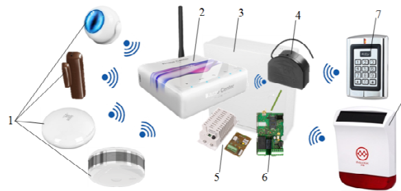
Fig. 1. Proprietary model: 1 – Z-Wave detectors; 2 – Fibaro HC Lite (switchboard); 3 – case; 4 – Fibaro relay FGS-211; 5 – backup power; 6 – GSM output; 7 – Z-Wave access keypad; 8 - Z-Wave alarm
